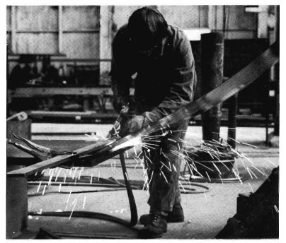
Coiled mild steel is unrolled and cut into 45 ft. lengths to form wagon sides.
