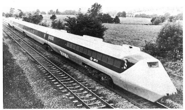
Britain's prototype Advanced Passenger Train (APT) on its first main line proving run prior to starting the most stringent test programme ever devised for a railway train. The APT project's objectives are to reduce journey time to a minimum by exploiting fully the potential of existing track and signalling equipment and provide superlative comfort at 155 m.p.h. (250kph). British trains at present have a maximum speed of 100 m.p.h. (160 kph). Photograph: London Press Service.
