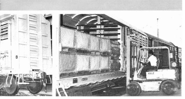
imental South Australian Railways wagon. Classed SL, it features two massive doors on each side which, when opened give rst visit to Melbourne, the wagon was loaded with nearly 20 tons of oranges from Loxton in South Australia for forwarding scacci said that the entire palletised load was unloaded by one fork lift truck in only 25 minutes. This was ideal for his company's loading.
