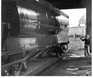
After coming off the assembly line, all wagons are sprayed with a de-oxidine to clean the metal ready for painting and inhibit rust.
