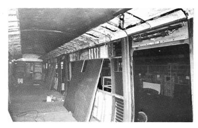
POLYURETHANE INSULATION lines the walls and ceiling, rubber insulation covers the floor to deaden under-carriage noise, and portion of the heating duct has been fixed to the roof. Also visible is the power-door mechanism and the walk-through arrangement at the rear of the carriage.
