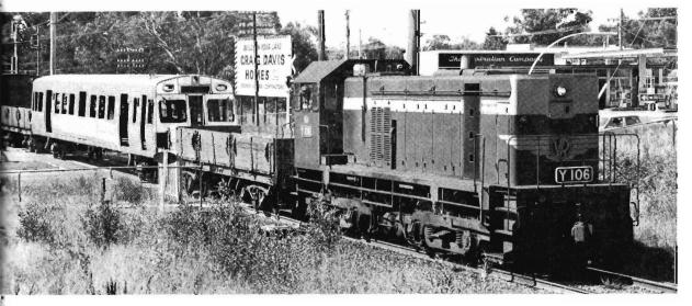
THINGS TO COME. Following its delivery to Bayswater station (see front cover), the shell of the first stainless steel the new metropolitan trains was placed on rail bogies, then taken to Martin & King's Somerton plant for fitting out.
