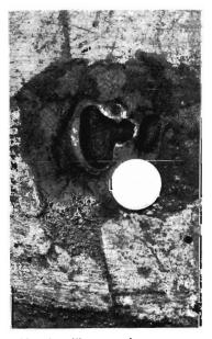
This ulcer-like corrosion on a gas pipe—larger than a 10c piece—was caused by electrolysis.
